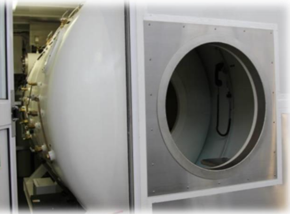
Air Dive Decompression Chamber
